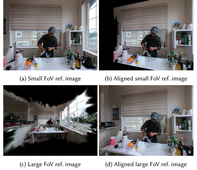
Fig. 8. Visualization of PRPA results with different reference FoVs. A small FoV (a) misses boundary content (b), whereas a large FoV (c) preserves coverage but reduces pixel density in the aligned reference image (d).
